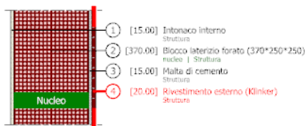
Figure 173: Perimeter wall with klinker cladding
