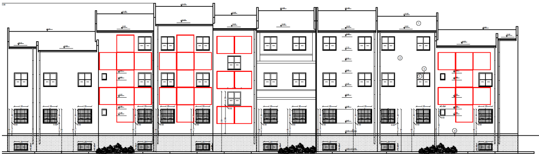
Figure 114. Installation of the ADBE technology on the building's south walls
