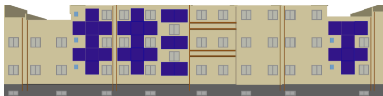
Figure 13: 3D design of the PV façade for the REHOUSE project in AutoCAD software
