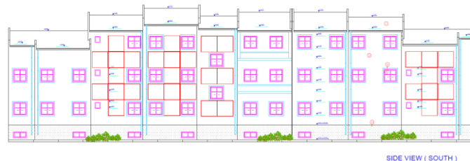
Figure 12: 2D design of the PV façade for the REHOUSE project in AutoCAD software
