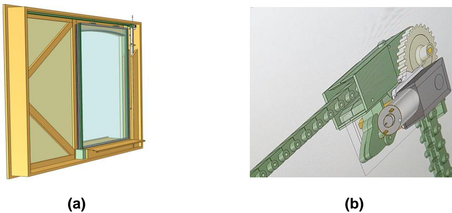
Figure 88. The IWS technology and its, (a) passive element (opening), (b) active element (solar thermal system)
