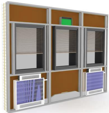
Figure 73. SmartWall conceptual view including BIPV, HVAC ducts, FCUs, batteries and smart blinds
