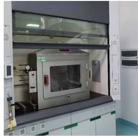
Figure 16: Single-flame source test
