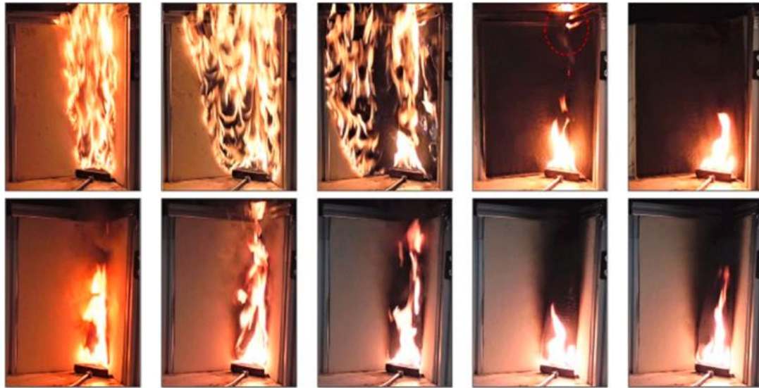
Figure 36: SBI test – Flames propagation
