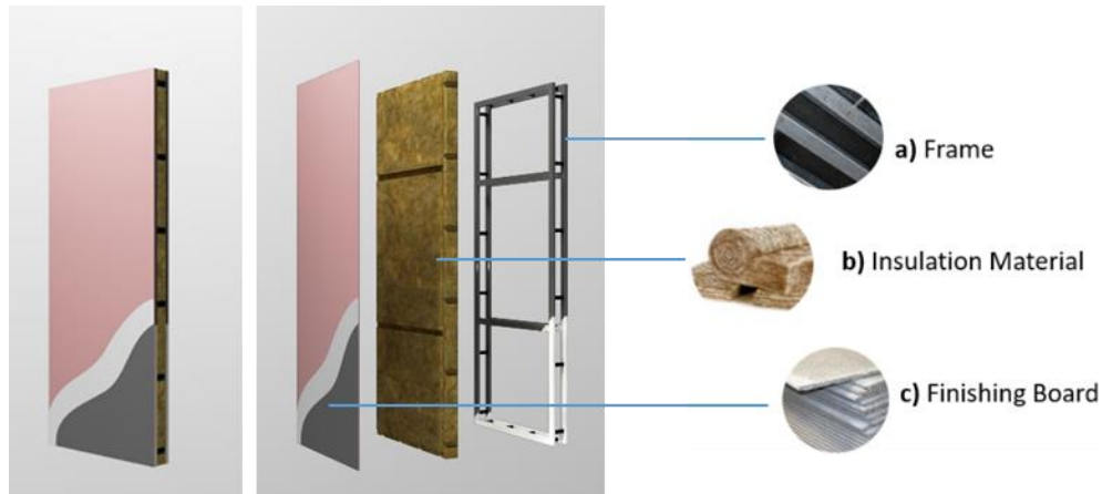
Figure 4: Basic Components of SmartWall Systems
