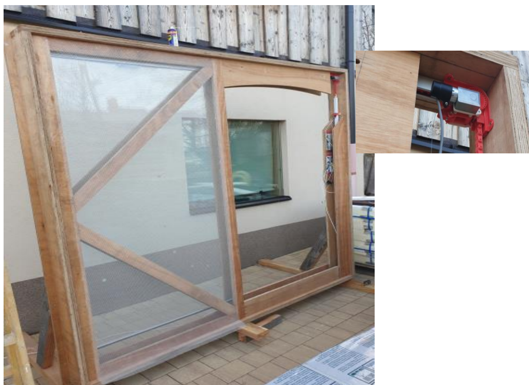
Figure 43: IWS life size prototype with the electric engine
