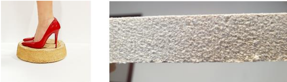
Figure 12: The activated cellulose insulation has a high compression strength
