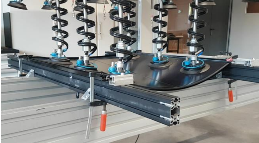
Figure 39: Mechanical load test – Equipment
