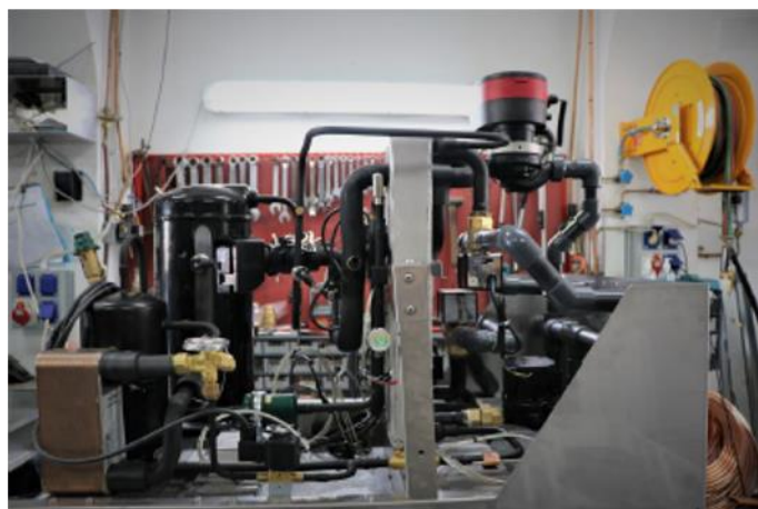
Figure 2: View of a designed multi-source heat pump with the main components
