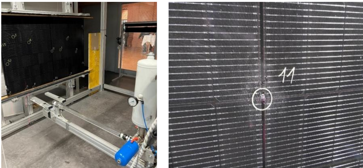
Figure 35: Hail resistance test – Equipment and module detail
