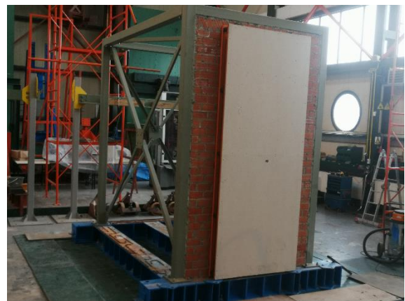
Figure 17: Earthquake shaking table with specimen
