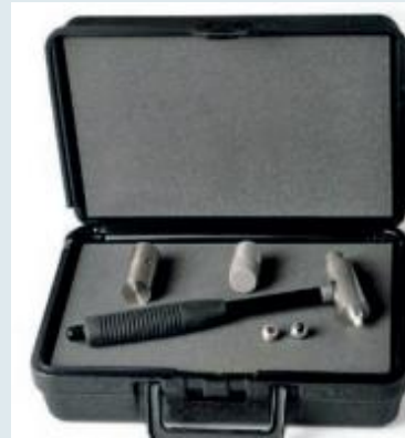
Figure 93: Sonic velocity instrumentation (instrumented hammer for measuring sonic velocity).
