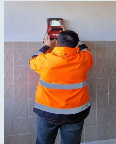
Figure 79: GPR scanning on the elevator case.
