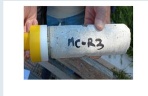
Figure 88: Thermo-hygrometric measurements on core.
