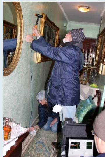
Figure 97: Execution of sonic test.
